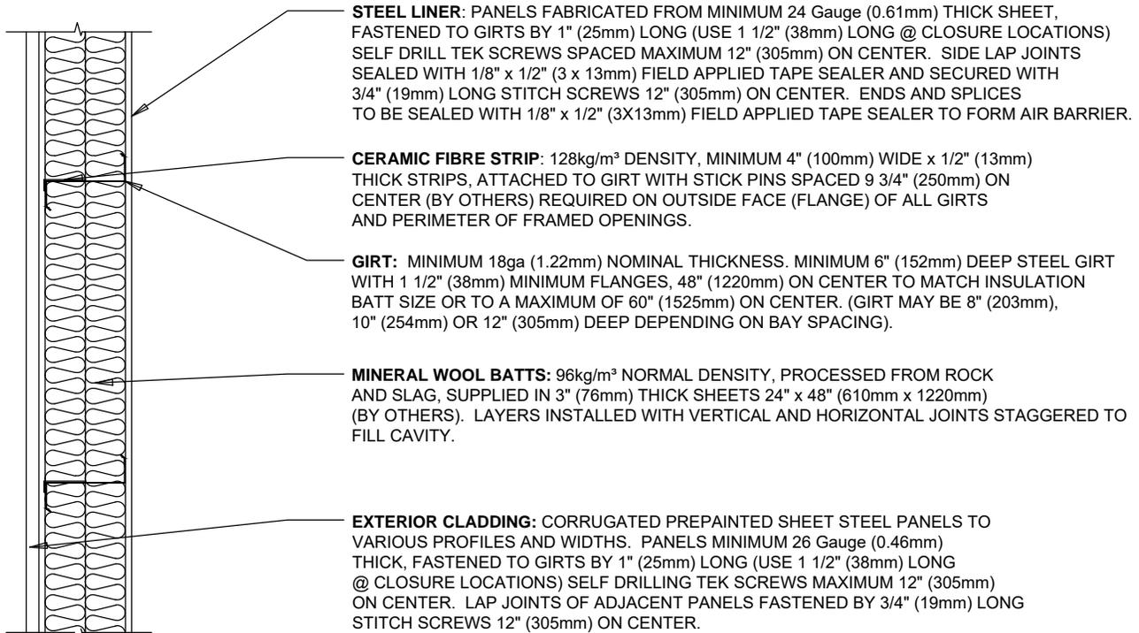
**TWO-HOUR FIRE RATED WALL ASSEMBLY (MEETS ULC DESIGN NO. W606)**
