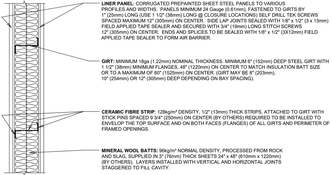
**TWO-HOUR FIRE RATED PARTITION WALL ASSEMBLY (MEETS ULC DESIGN NO. W611)**
