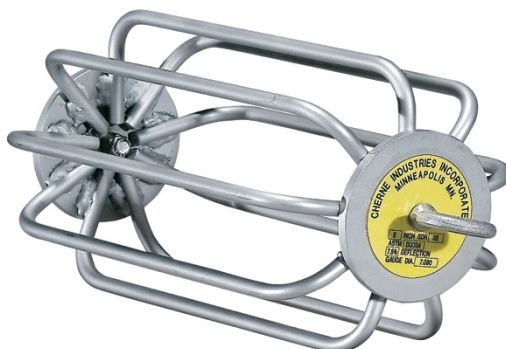
FIGURE 1: Typical mandrel (ref. Cherne Industries, Incorporated)
